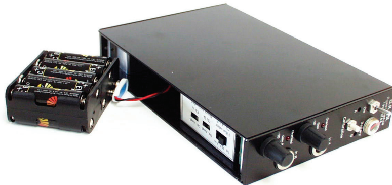
Fig. 3.1 Showing the battery pack of the Power Module Type 12AA
